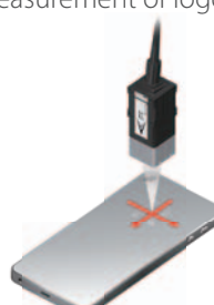
Level difference measurement of logos
