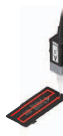
Flatness measurement of cover glass by itself
