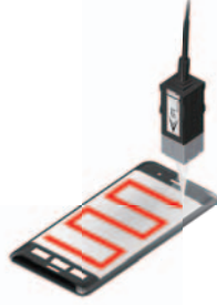
Flatness measurement of cover glass
